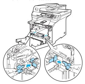
Put a piece of paper (letter or A4) on the belt unit to prevent damage to the belt unit.
